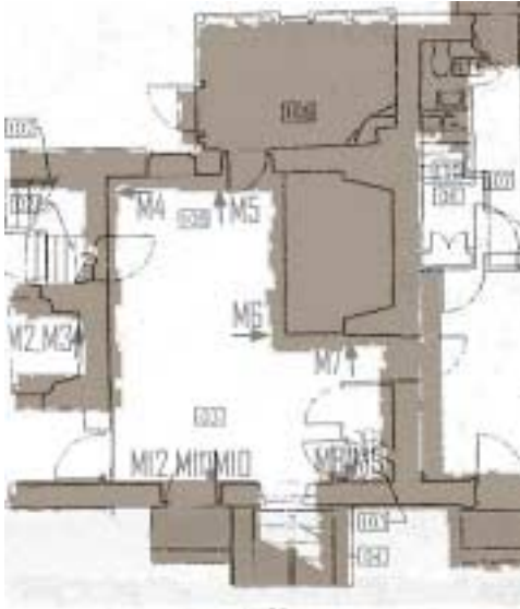
Unit "B" cellar (brown) with black outline overlay of 1 st floor. Cellar Mortar sample locations marked. Old retaining wall along east end of "B" visible in this diagram and as N-S running ledge in "C0" kitchen.
